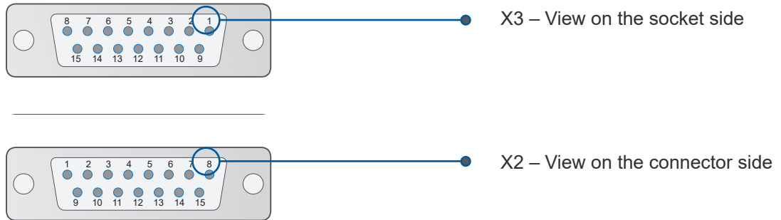
Image 5: PIN-assignment of Plugs and Sockets
