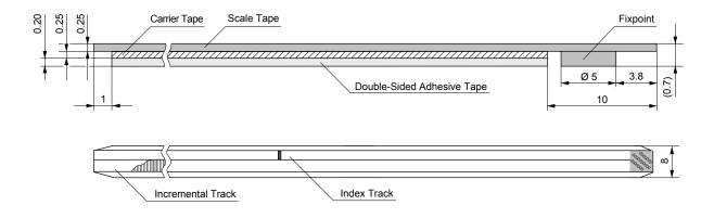
The two steel tapes are uncoupled mechanically. This ensures that the upper steel tape can expand independently of the lower steel tape due to thermal variations of the ambient temperature. By reference of the ambient temperature and the expansion coefficient of the steel tape it is possible to determine occurring length deviation of the increments. This allows you to substract out the deviation of the measurement results.
